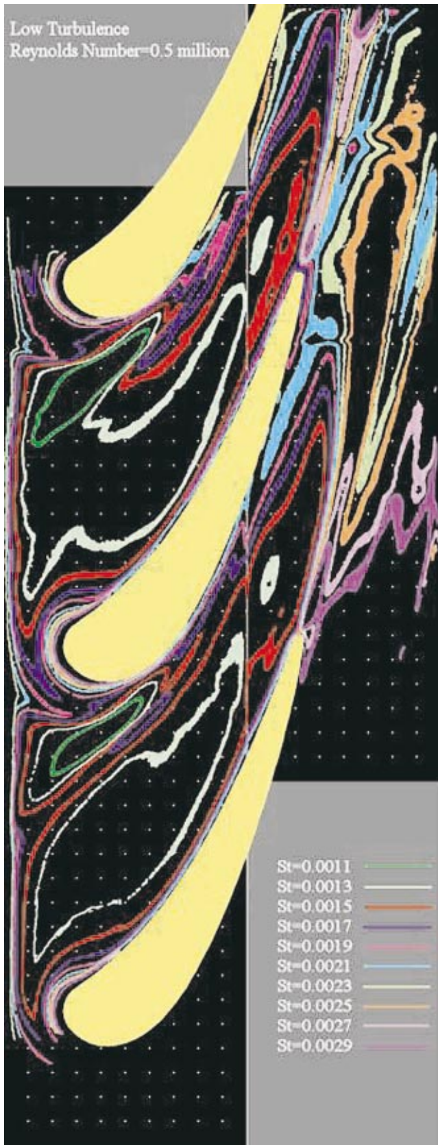
Fig. 9 Endwall Stanton number contours, LT, Tu=0.007 , Re_c=500,000
