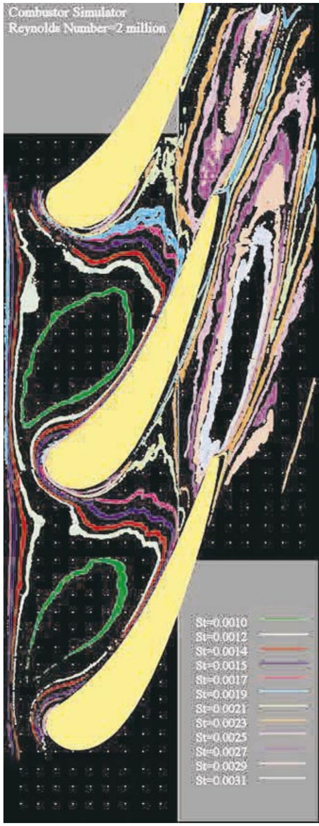
Fig. 14 Endwall Stanton number contours, AC, Tu=0.134 , Lu=7.3 cm, Re_c=2,000,000
