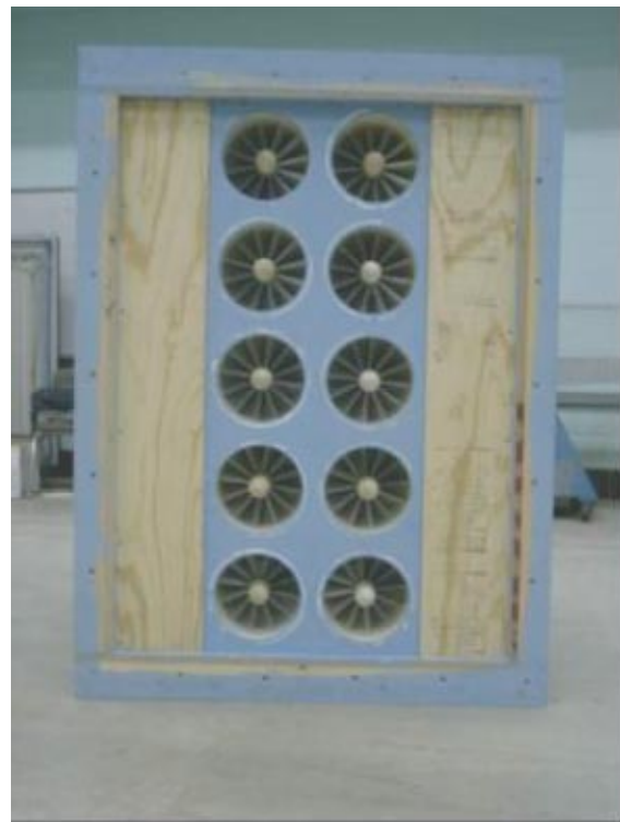
Fig. 4 Digital photo of dry low \text{NO}_x swirlers installed in mock combustor liner
